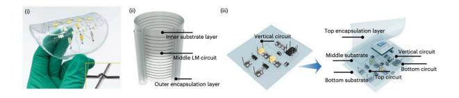
Flexible electronics prepared using 3D structured Ga–10In solid wire: flexible LED array with arched interconnects (i), wearable 3D structured finger movement detection sensor (ii) and multilayer flexible circuit board (iii). Credit: Li et al. (Nature Electronics, 2023).
