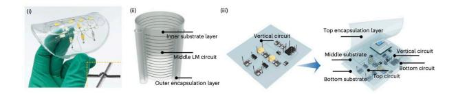
Flexible electronics prepared using 3D structured Ga–10In solid wire: flexible LED array with arched interconnects (i), wearable 3D structured finger movement detection sensor (ii) and multilayer flexible circuit board (iii). Credit: Li et al. (Nature Electronics, 2023).
