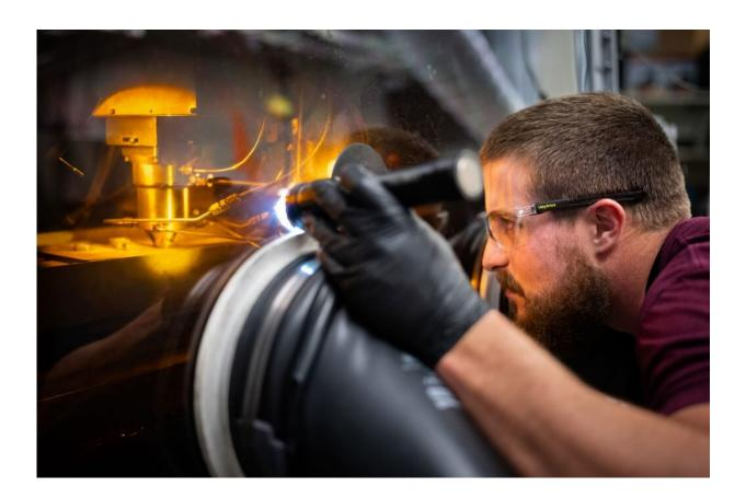
Sandia technologist Levi Van Bastian works to print material on the Laser Engineered Net Shaping machine, which allows scientists to 3D print new superalloys. Credit: Craig Fritz
