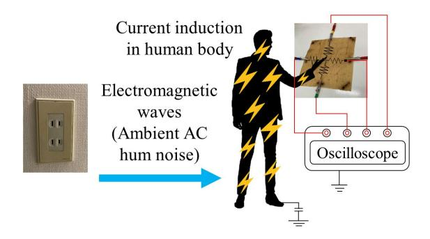
Electromagnetic waves from everyday power sources induce small currents inside the human body. This can leak out when we touch surfaces. A set of electrodes and an oscilloscope can detect these currents and locate where on the surface was touched. The process requires calibration to correctly convert currents into locations. Credit: Tokyo Metropolitan University
