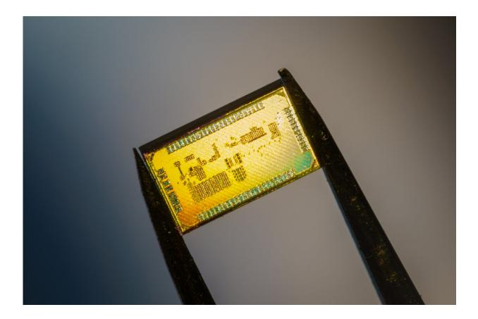
The custom chip, which is roughly the size of a grain of sand and costs only a few pennies to manufacture, needs so little power that it can be entirely powered by LTE signals, a technique called RF energy harvesting. Credit: David Baillot/University of California San Diego
