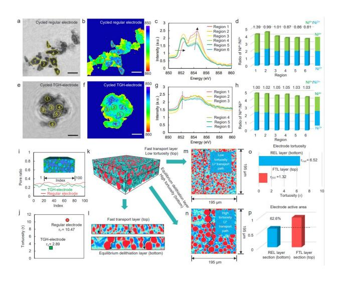
(a) Ptychography STXM amplitude (optical density) image and (b) elemental distribution mapping at the Ni edges of cycled regular cathodes. (c) XAS spectra of the Ni L3-edge and (d) quantification of the Ni<sup>3+</sup> and Ni<sup>4+</sup> in different regions. (e) Ptychography STXM amplitude (optical density) image and (f)
