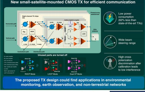
A Small-Satellite-Mounted 256-Element Ka-Band CMOS Phased-Array Transmitter Achieving 63.8dBm EIRP Under 26.6W Power Consumption Using Single/Dual Circular Polarization Active Coupler
