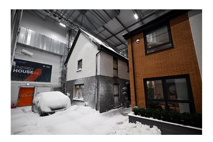
Simulated snow covers a car and the walls of one of two houses built in a lab to develop future heating solutions that will use less energy and help meet climate goals.
