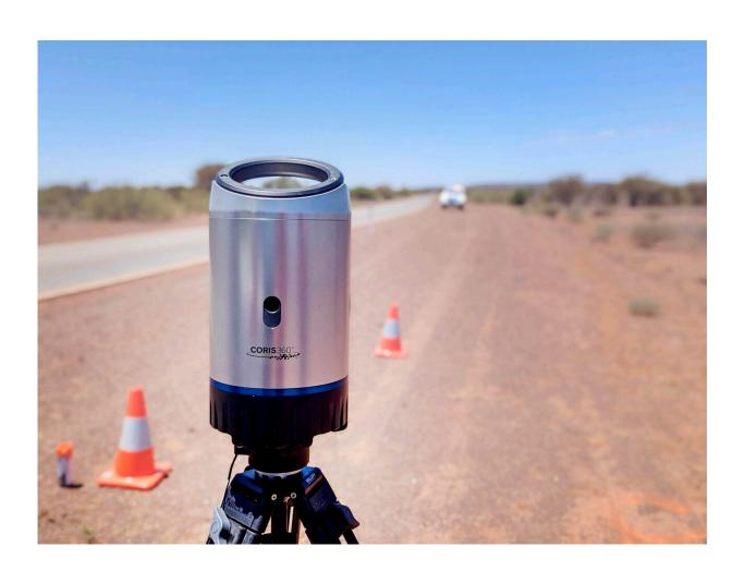
The Coris360 imaging technology on the road in Western Australia to locate a radioactive source. Credit: ANSTO
