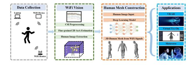
Wi-Mesh analyzes the wi-fi signals reflections at multiple antennas to construct 3D human mesh representation, which can then be utilized for various innovative applications. Credit: Yichao Wang and Jie Yang
