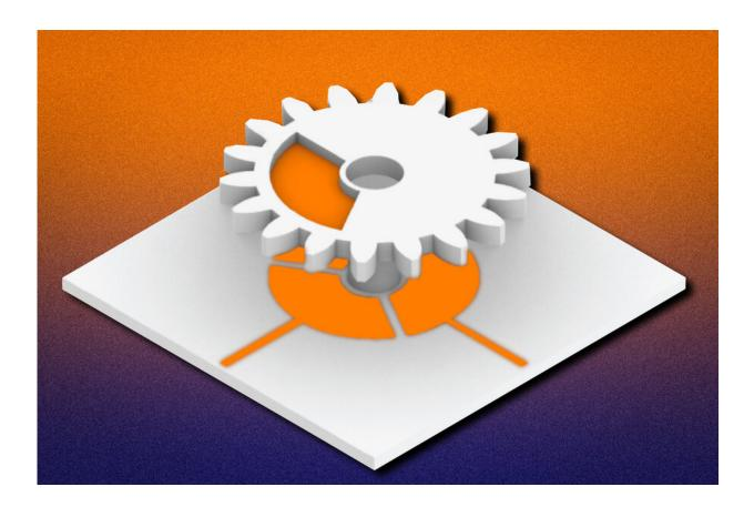
MIT researchers created a system that enables makers to incorporate sensors directly into rotational mechanisms with only one pass in a 3D printer. This gives rotational mechanisms like the gears inside a motor the ability to sense their angular position, rotation speed, and direction of rotation. Credit: Massachusetts Institute of Technology
