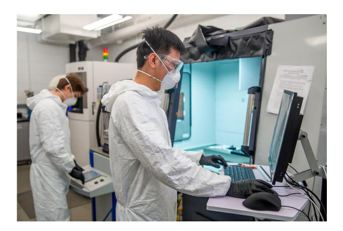
The metal 3D printers used by U of T Engineering Professor Yu Zou and his team are designed to specialize in both selective laser melting and directed energy deposition—two essential metal additive manufacturing techniques. Credit: Safa Jinje
