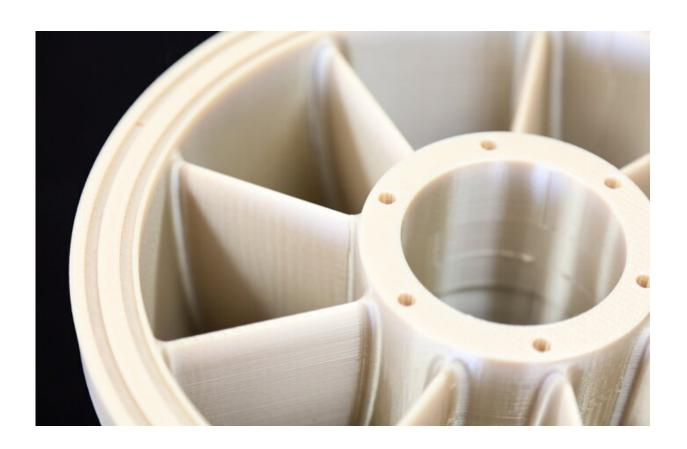
This newly manufactured fixed guide vane of a hydropower turbine system was additively created at the DOE Manufacturing Demonstration Facility at ORNL. Credit: Genevieve Martin/ORNL, U.S Dept. of Energy
