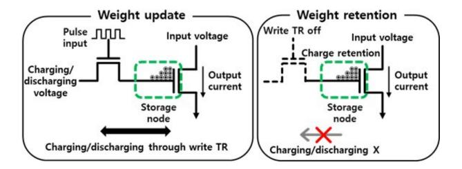
AI synaptic device operation using oxide semiconductors. The conductance of the read transistor can be controlled by charging/discharging the storage node
