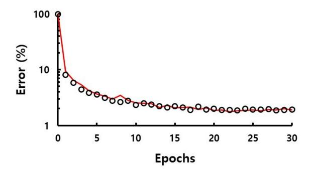
Simulation results of MNIST classification using IGZO 2T synaptic devices. High linear and symmetric weight programming characteristics of AI synaptic devices based on oxide semiconductors enable accurate training processes that minimize errors in artificial intelligence systems. In a simulation of random handwriting recognition, these devices achieved an inference accuracy of approximately 98%, which is nearly identical to the accuracy of ideal mathematical calculations. Credit: POSTECH
