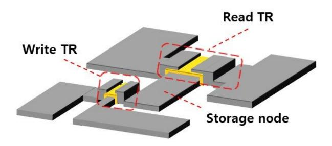
Structure of the proposed AI synaptic device. Two oxide semiconductor transistors are connected; one for writing and the other for reading. Credit: POSTECH
