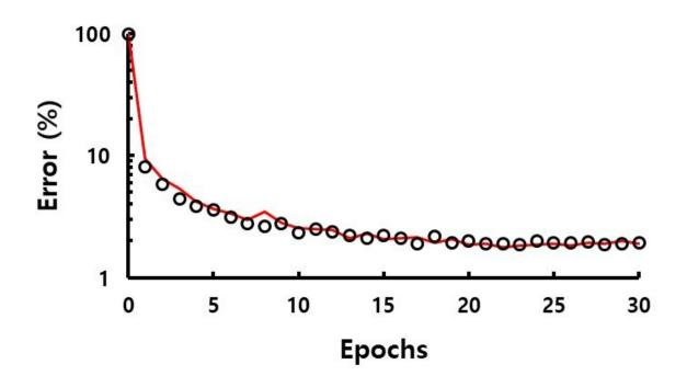
Simulation results of MNIST classification using IGZO 2T synaptic devices. High linear and symmetric weight programming characteristics of AI synaptic devices based on oxide semiconductors enable accurate training processes that minimize errors in artificial intelligence systems. In a simulation of random handwriting recognition, these devices achieved an inference accuracy of approximately 98%, which is nearly identical to the accuracy of ideal mathematical calculations. Credit: POSTECH
