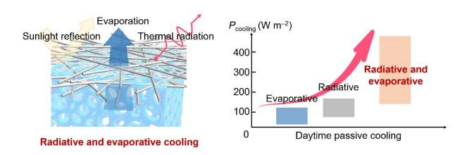
Scientists from Tsinghua University develop an integrated radiative and evaporation cooling technology by using an evaporative hydrogel and permeable radiative cooling layer to achieve cooling. Credit: Nano Research Energy, Tsinghua University
