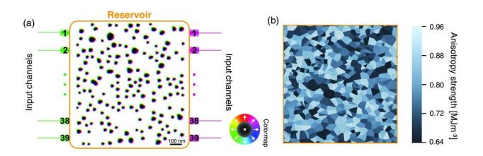
a) Schematic of a multicontact skyrmion reservoir with 39 electrical contacts on each side. The dark points represent skyrmion cores and the cyclic colormap around them represents the orientation of in-plane magnetization. Contacts have been enlarged for visibility. b) Random grain distribution underlying the skyrmion reservoir. Each grain has a particular anisotropy strength.
