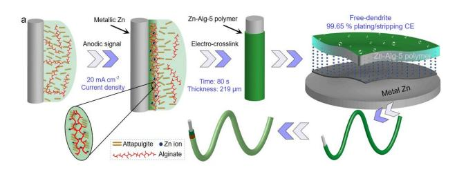
The schematic illustration of in-situ preparation procedure, properties, and construction of Zn-Alg-5 polymer electrolyte using a wire-shaped Zn electrode for a Zn battery. Credit: Science China Press
