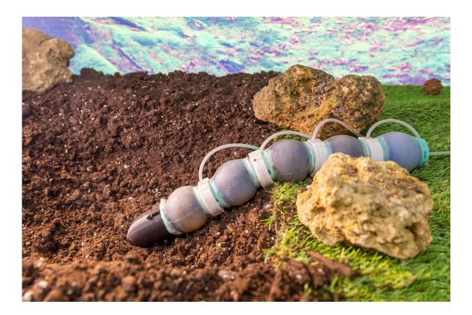
The creation of earthworm-like robot was made possible through a thorough understanding and application of earthworm locomotion mechanics. The current prototype is 45 cm long and weighs 605 grams. Created by researchers at Italian Institute of Technology in Genoa, Italy. Credit: IIT-Istituto Italiano di Tecnologia
