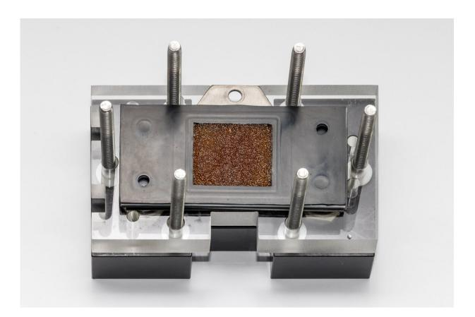
View into the cell stack: a low-cost electrolyte made of synthetic resin provides the cell with additional stability. Credit: Forschungszentrum Jülich / Ralf-Uwe Limbach
