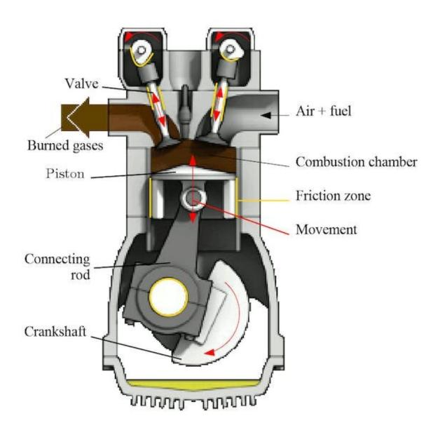
Diagram of a combustion engine: movement of parts (red) and friction areas (yellow). Credit: Zephyris/Wikimedia/TCF, <u>CC BY</u>
