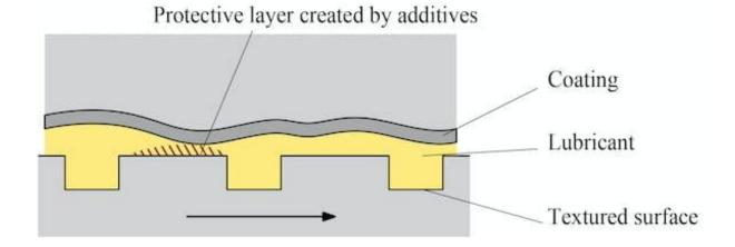
Solutions used to reduce friction and wear in mechanical contact areas. Credit: Zephyris/Wikimedia/TCF, <u>CC BY</u>
