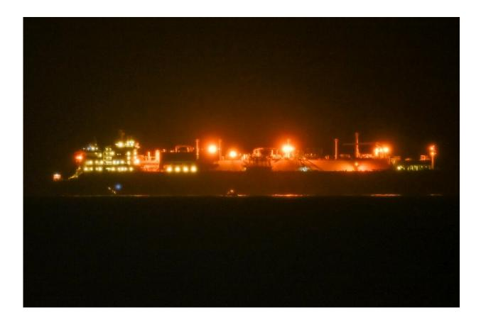
The Golar Tundra will receive liquified natural gas (LNG) from other carriers, which it will turn back into a gaseous state that can be fed into Italy's national network.
