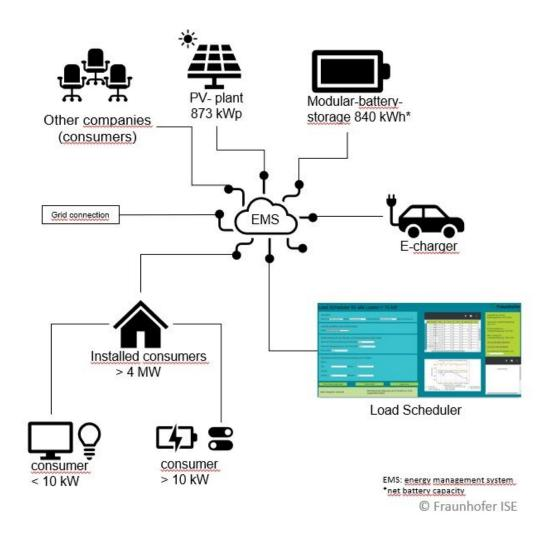
The Haid Power project's intelligent energy and load management systems regulate energy supply and combine electricity from battery storage with electricity from the public grid. Credit: Fraunhofer-Gesellschaft
