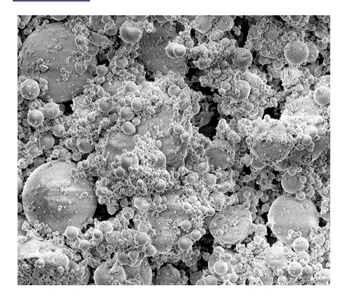
Heavy-metal-free coal fly ash improves cement strength and flexibility. Credit: Rice University.
