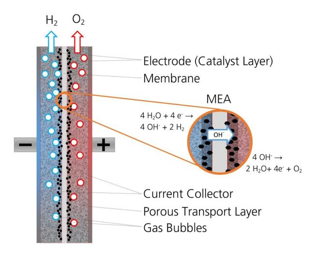
Diagram of an AEM electrolysis cell: The key element is the membrane electrode assembly (MEA), which consists of the anion-conducting membrane and the directly connected electrodes. Credit: Fraunhofer-Gesellschaft
