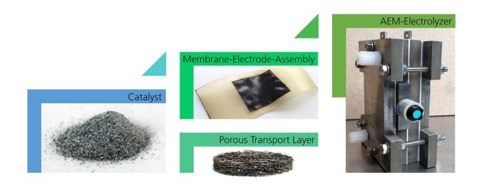
Fraunhofer IFAM is working with German and New Zealand partners in the HighHy project to develop highly active catalyst materials and incorporate them into a membrane electrode assembly. Credit: Fraunhofer-Gesellschaft
