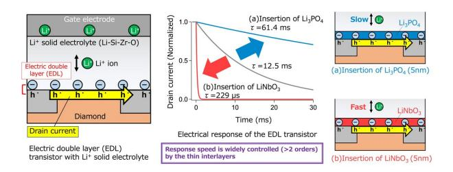
Investigating the EDL effect at the solid electrolyte interface by a novel technique, researchers tuned switching response time and achieved carrier modulation at the interface between a hydrogen-terminated diamond (H-diamond) and a Li<sup>+</sup>-conducting solid electrolyte/solid interface. Credit: Tohru Higuchi from Tokyo University of Science
