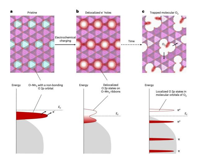
a–c, Structural schematics illustrating the pristine structure (a) the charged structure with delocalized electron holes on O–Mn2 (b) and a charged structure after condensation of the delocalized holes to form molecular O2 (c). Below each structure are schematic density of-states plots illustrating the changes to the
