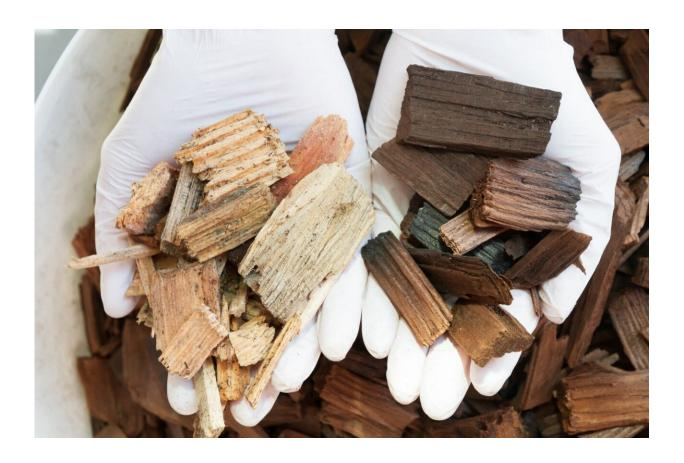
Beechwood chips torrefied with superheated steam (right) have an increased calorific value compared to untreated chips (left) and moreover are hydrophobic. Credit: Fraunhofer IGB
