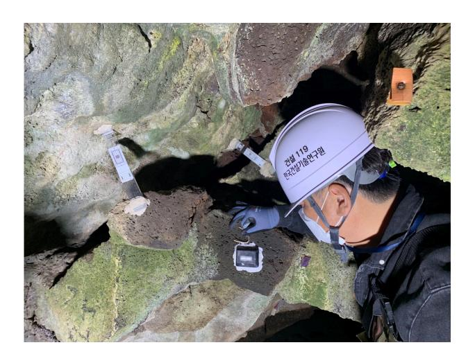
Photo of the site attaching the developed sensor in the lava cave. Credit: Korea Institute of Civil Engineering and Building Technology
