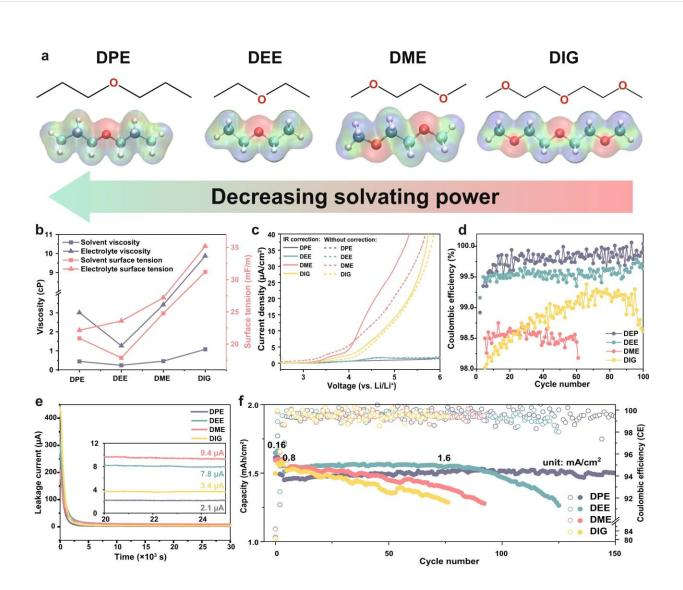
All the electrolytes contain 1.8 M LiFSI salt, all the tests were performed at 25 °C. **a** The electrostatic potential (ESP) maps of the studied ether molecules. The
