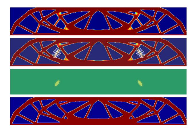
This sequence shows an example of the iterative design process in action. On top, you can see the AI-designed initial version of a support beam. In the second and third images, a human operator highlights two support segments as unnecessary. The bottom image shows how the AI system incorporates that input by eliminating those segments and strengthening others to compensate. Credit: MIT News.
