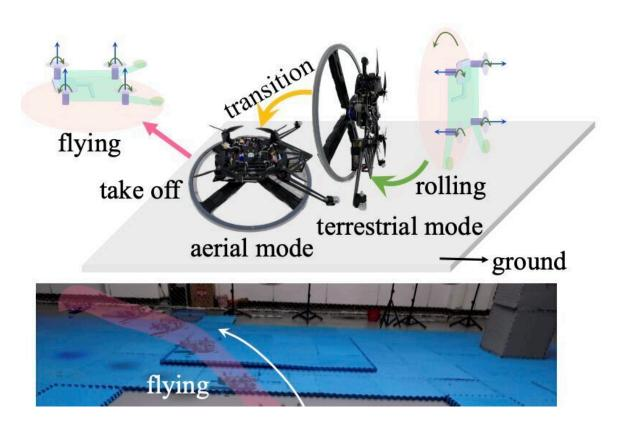
The vehicle created by the researchers and its different modes of operation. Credit: Zheng et al
