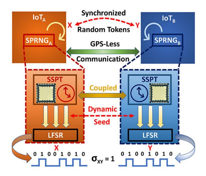
The concept of GPS-free secure Communication in spatially separated IoTs with SPRNGs: The IoTs generate random tokens using the SPRNG for use as cryptographic keys. The tokens are generated using a combination of a fast, low-complexity LFSR seeded by the Secure self-powered timers (SSPT). The synchronization of SSPT across both  $IoT_A$  and  $IoT_B$  ensures that the random
