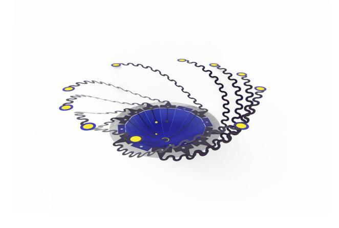
FEA result of a 3D electronic cell scaffold: A 3D assembled electronic cell scaffold based on the microlattice design. Credit: Prof. Yihui Zhang (Tsinghua University)
