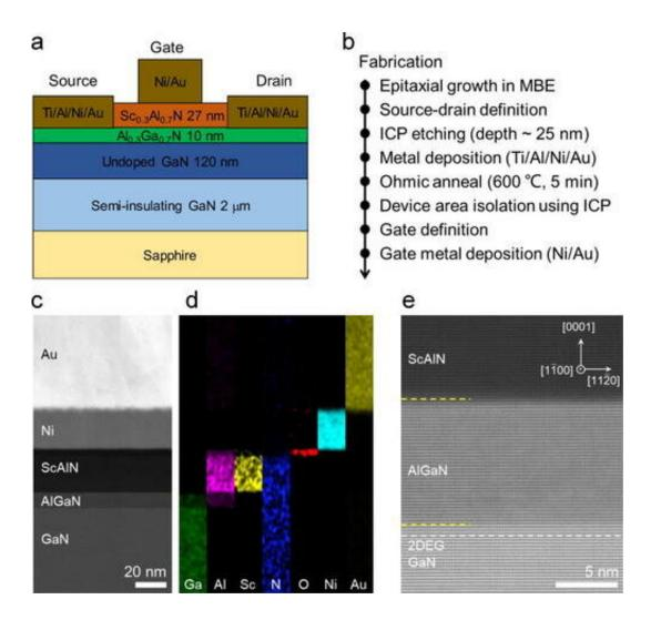
(a) Schematics of the epitaxial ferroelectric HEMT device structure. (b) Main fabrication steps. (c) HAADF-STEM image captured from the gate stack region and (d) corresponding EDS mapping showing the element distribution. (e) High resolution HAADF-STEM image showing the atomic stacking at the heterostructure interfaces. Credit: *Applied Physics Letters* (2023). DOI:
