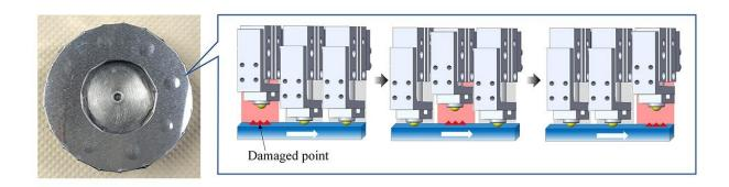
How to avoid contact with damaged position using morphing surfaces. Credit: Motoyuki Murashima
