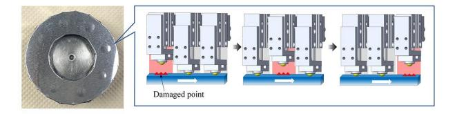
How to avoid contact with damaged position using morphing surfaces. Credit: Motoyuki Murashima
