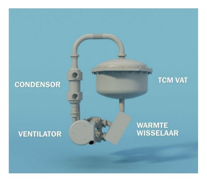
The salt battery consists of four components linked in a closed system. Credit: Jelle Houben
