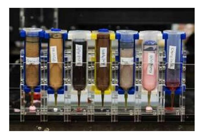
3D-printing system that constructs a dish comprising seven ingredients, cooked in situ using a laser. Credit: Jonathan Blutinger/Columbia Engineering
