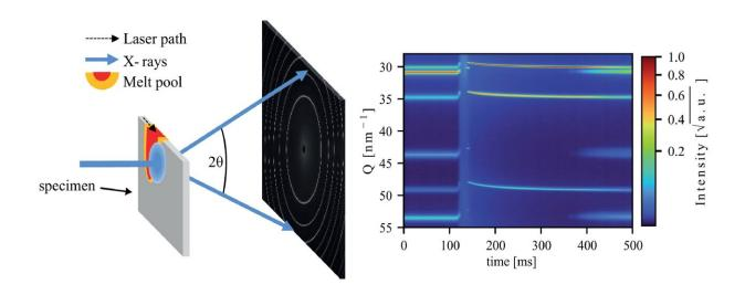
Researchers used high-speed X-ray diffraction to identify the crystal structures that form within steel as it is 3D-printed. The angle at which the X-rays exit the metal correspond to types of crystal structures within. Credit: H. König et al. via Creative Commons, adapted by N. Hanacek/NIST
