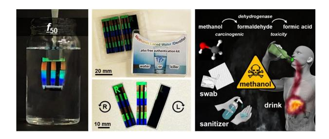
Development of the kit to detect methanol contamination in water. Credit: Korea Institute of Science and Technology
