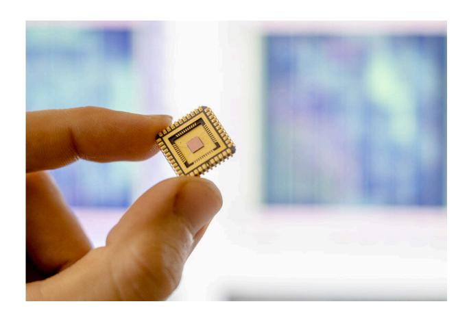
For their project, the researchers took thousands of microscopic images of microchips. Pictured here is such a chip in a golden chip package. The chip area that was inspected only measures about two square millimetres. Credit: RUB, Marquard
