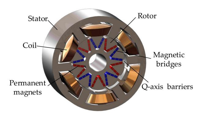
Structure of a reverse-salient permanent magnet synchronous motor analyzed in a separate study. Credit: *Machines* (2022). DOI: 10.3390/machines10030204
