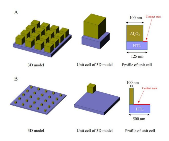
Schematic representation of 2D PIC model simplified from 3D periodical structure for dielectric width d=100 nm with a spacing of (A) 25 nm and (B) 400 nm. Arrow indicates the contact area (opening area) between perovskite and
