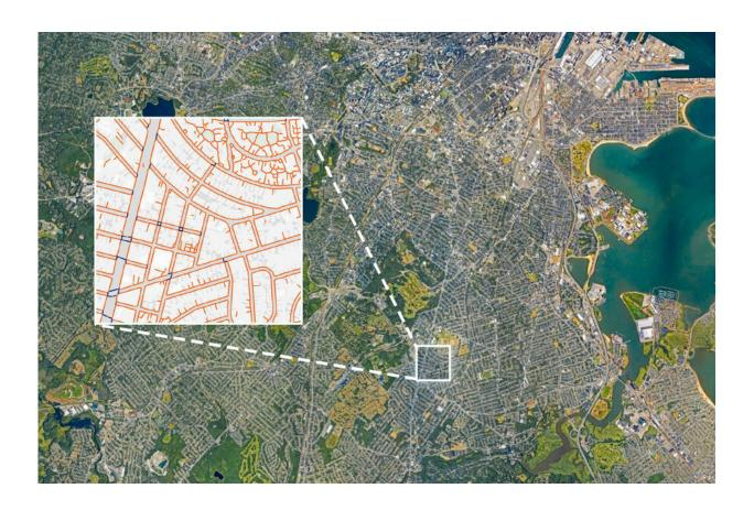
MIT researchers have built TILE2NET, an open-source tool that uses aerial imagery and image-recognition to create complete maps of sidewalks and crosswalks. Pictured is a view of Boston with an inset showing how the model detected sidewalks, crosswalks, and footpaths. Credit: Inset courtesy of the researchers. Background via Google Earth
