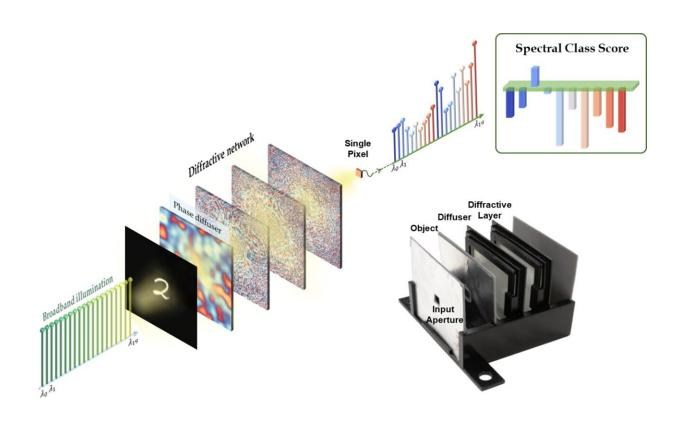
The single-pixel broadband diffractive neural network classifies handwritten digits through unknown random diffusers. A broadband single-pixel diffractive optical network maps the spatial information of input objects behind an unknown random diffuser into the power spectrum at the output pixel aperture. Spectral class scores reveal the type of input object behind the random diffuser. Credit: Ozcan Lab @ UCLA.
