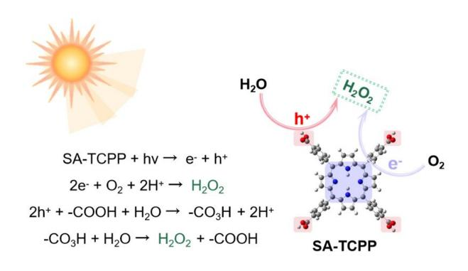
The proposed schematics for H<sub>2</sub>O<sub>2</sub> production on SA-TCPP supramolecular photocatalysts. Credit: Zhang et al
