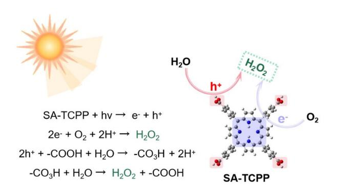
The proposed schematics for  $H_2O_2$  production on SA-TCPP supramolecular photocatalysts. Credit: Zhang et al
