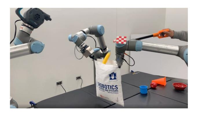
The self-supervised learning framework Columbia Engineers call DextAIRity learns to effectively perform a target task through a sequence of grasping or airbased blowing actions. Using visual feedback, the system uses a closed-loop formulation that continuously adjusts its blowing direction. Credit: Zhenjia Xu/Columbia Engineering
