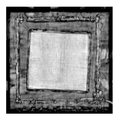
Radar images (co-polarization) of a fiber layer package with non-visible undulation below the surface. Credit: Fraunhofer-Gesellschaft
