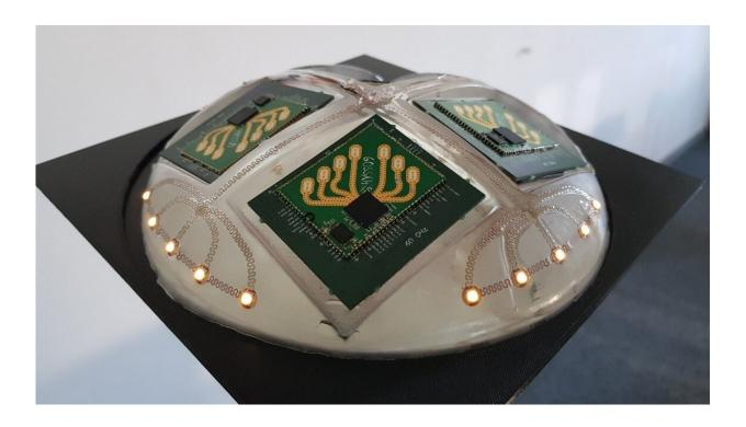
The polyurethane ceiling unit equipped with four radar modules. Credit: Fraunhofer-Gesellschaft
