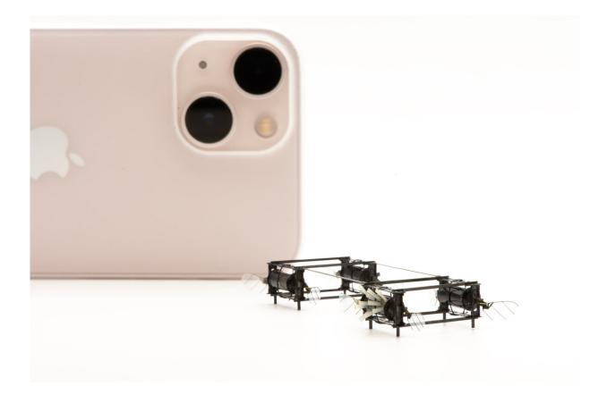
The insect-scale aerial robot and its actuators. Credit: Yi-Hsuan Hsiao
