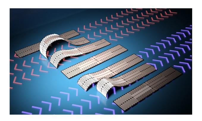
Researchers at North Carolina State University have demonstrated a caterpillar-like soft robot that can move forward, backward and dip under narrow spaces. The caterpillar-bot's movement is driven by a novel pattern of silver nanowires that use heat to control the way the robot bends, allowing users to steer the robot in either direction. Credit: Shuang Wu, NC State University
