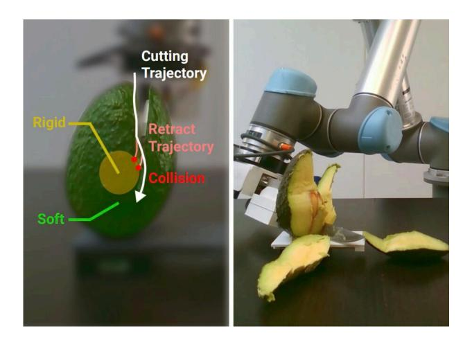
RoboNinja is designed to cut multi-material objects with an interactive state estimator and adaptive cutting policy. Left: When the knife encounters a collision with the invisible core, the algorithm updates the core estimation and replans the cutting trajectory after a few retracting actions. Right: We deploy the learned model on a physical robot, allowing it to cut fruits in a way that maximizes the cut-off mass while minimizing collision occurrences. Credit: Xu et al
